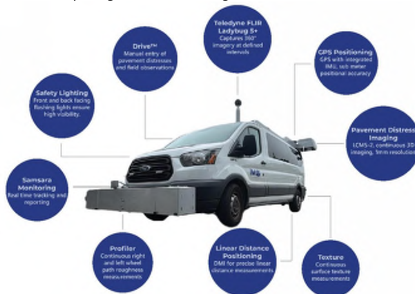
Figure 6 – LCMS-2 data collection vehicle
